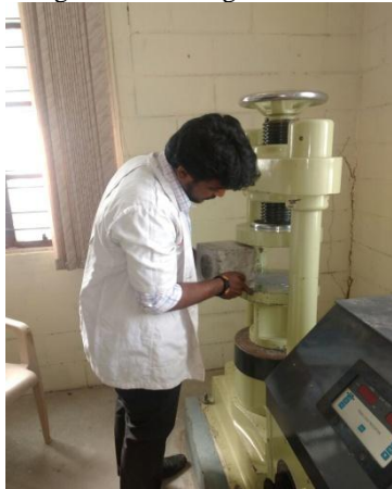
Figure 7– Compressive Testing of Cubes
